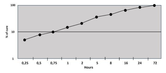
The graph shows the rate of cure for a M10
