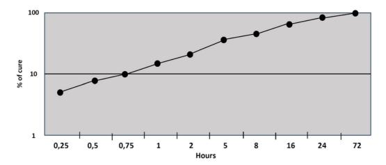
The graph shows the rate of cure for a M10
